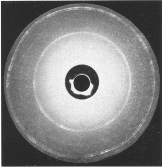
Figure 7 X-ray back reflection pattern of alloy C fractured in slow tension at 100°C.
